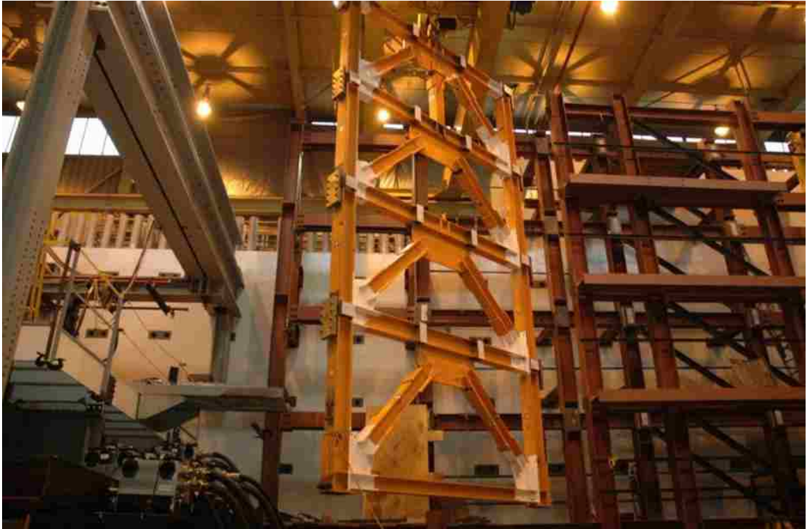
Figure 2.11: 60% scaled 4-story SC-CBF frame being removed from test setup after the experiments, from [66]
